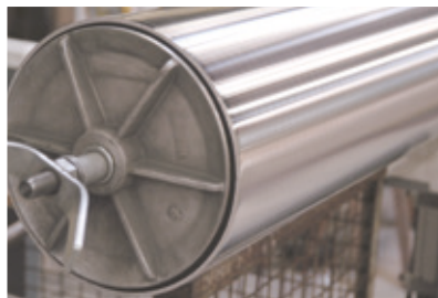
All pipes received a special surface grinding
