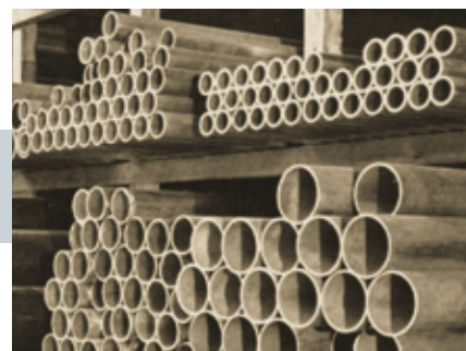
1890 Transition from handcraft to industrial operation (mass production of soldered copper pipes)
